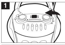
Open the CD compartment by pressing the CD Door OPEN/ CLOSE area. Place a disc on the spindle, label side up, and close the CD compartment door.
